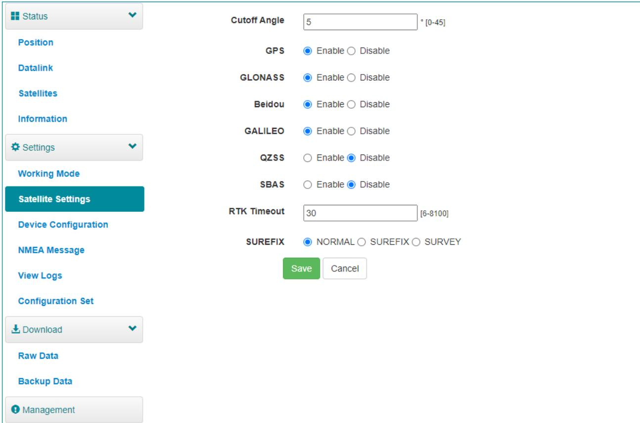
The screenshot displays the 'Satellite Settings' page. On the left is a navigation menu with categories: Status, Position, Datalink, Satellites, Information, Settings (expanded), Working Mode, Satellite Settings (highlighted), Device Configuration, NMEA Message, View Logs, Configuration Set, Download, Raw Data, Backup Data, and Management. The main content area includes:
