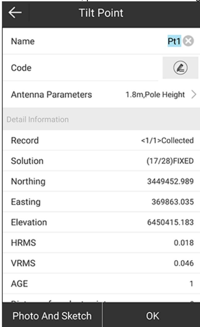
The screenshot shows a mobile application interface for a 'Tilt Point'. At the top, there is a back arrow and the title 'Tilt Point'. Below the title are several input fields: 'Name' with the value 'Pt1', 'Code' with an edit icon, and 'Antenna Parameters' with the value '1.8m,Pole Height'. A section titled 'Detail Information' contains a table with the following data:
