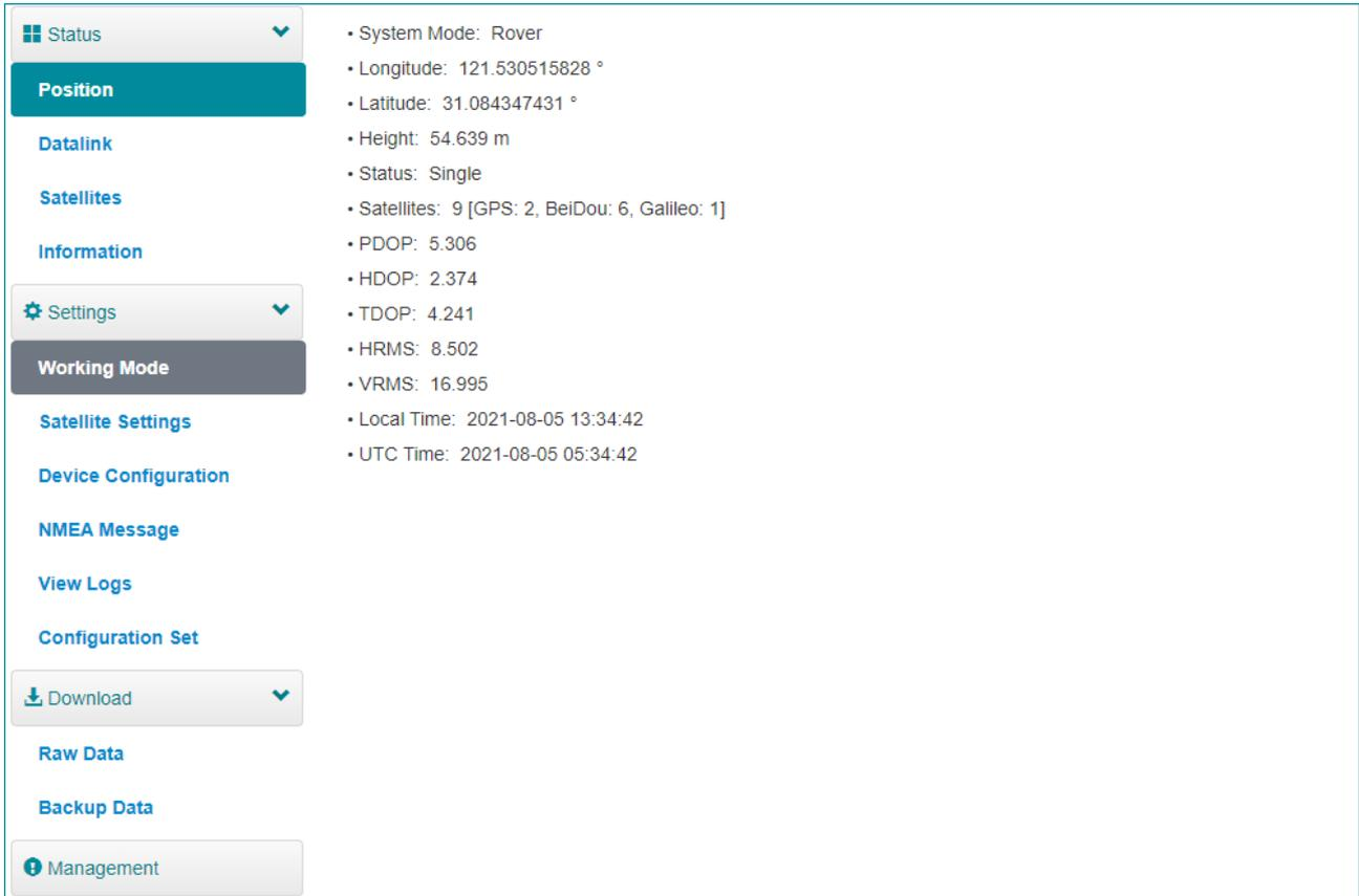
The screenshot shows a web interface for the Position page. On the left is a sidebar with navigation options: Status (selected), Position, Datalink, Satellites, Information, Settings, Working Mode, Satellite Settings, Device Configuration, NMEA Message, View Logs, Configuration Set, Download, Raw Data, Backup Data, and Management. The main content area displays the following data:
